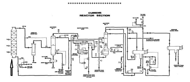
REACTOR IS UP FLOW WITH SINGLE FEED POINT AT BOTTOM
