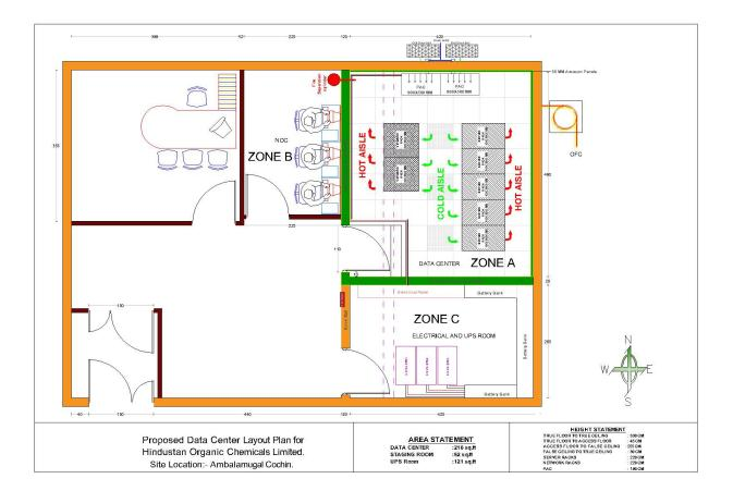
**Zone A** - This DC Server room area would host servers, server racks, storage racks, networking component Racks, and AHU, The area of Zone A is approximately be 220sqft.
